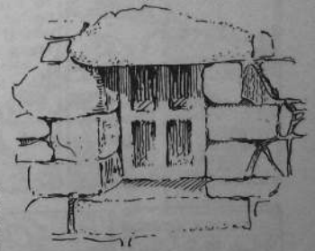
Window openings are traditionally made with a large granite lintel above and below the window.
