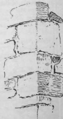
Corners derive their strength from being made out of cut, granite stones which fit together without the need for cement.
