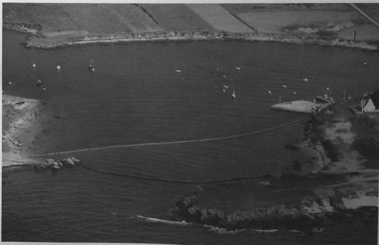
6-26. In the early stages of the spill, booms were not effective. However, booms deployed later across some harbor entrances and adequately tended reduced the amount of oil entering these systems.
