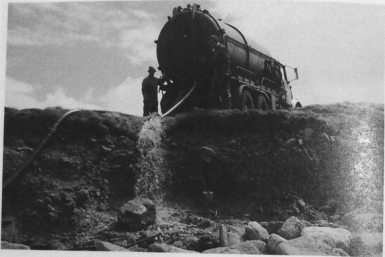
6-19. A vacuum truck decants water collected along with the oil. Much effort was lost early in the spill by failure to properly decant tankage.
