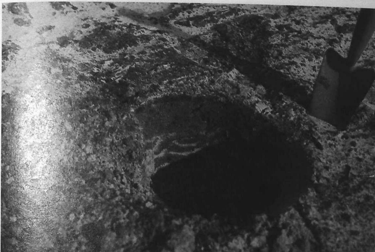
6-25. Close-up of the oiled sands at St. Michel-en-Greve. Shown are the oiled sand at the surface and the various oiled sand layers that have resulted from the deposition of sand and oil since the oil first reached this spot.
