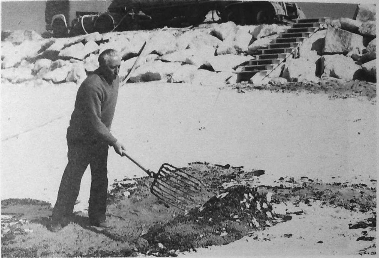
6-29. The use of plaster as an absorbent material was tried on a coarse beach near Tregastel. Several other techniques using rubber absorbents, peat, and other fibrous materials were also tested.
