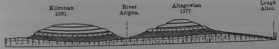
Fig. 33. Section through the Leitrim Coalfield showing the Coal Measures resting on the "Millstone Grit" and underlying shales and, below, the Carboniferous Limestone. (After E. Hull.)
