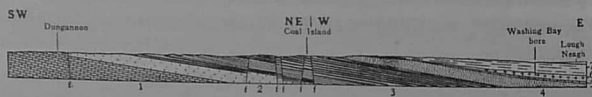
Fig. 30. Section through the Coal Island Coalfield and Washing Bay boring. 1. Carboniferous Limestone; 2. "Millstone Grit"; 3. Coal Measures; 4. Trias; 5. Chalk; 6. Tertiary basalt-lavas; 7. Lough Neagh Clays; f, fault.
