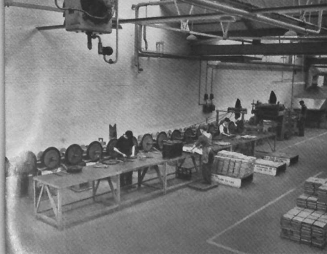
Pay-off End of Export Strap Blueing Line at the works of Signode Ltd., Swansea.
