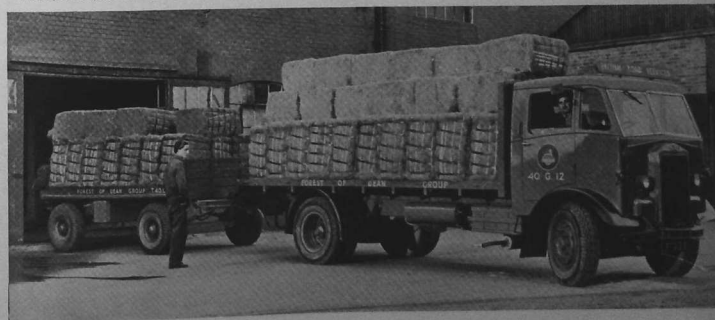
A Vehicle and Trailer for General Purposes, where body space rather than dead weight is required.
