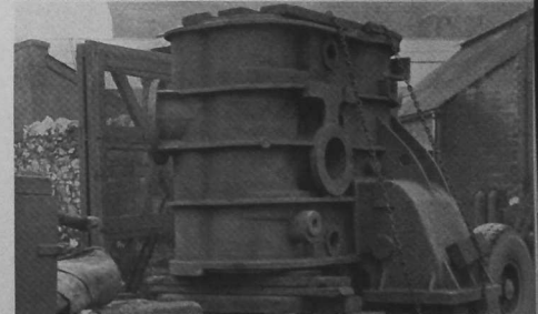
High Pressure Cylinder Block Casting weighing nearly 10 tons, specially manufactured for a Marine Engine by Tubal Cain Foundry & Engineering Works Limited, Cardiff.
