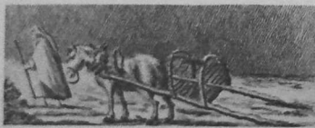
Sledges like this could be pulled over the roughest roads. But they did not last long and could only carry very small loads
