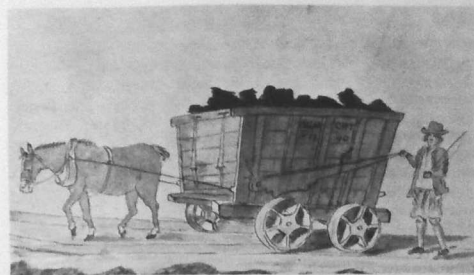
A coal wagon being pulled along a wooden wagonway. The man at the back was needed to whip the horse up hills, and put the brake on when going downhill
